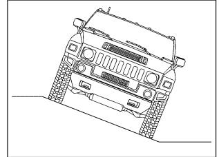
Also, your vehicle should be able to traverse a 40% (22 degrees) side slope at 6 mph (9.7 km/h) while fully loaded on high friction surfaces.
